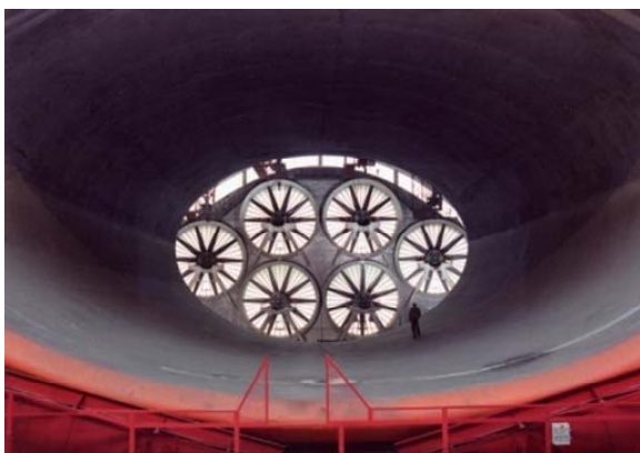
Figure 5 The diffuser of the large Wind Tunnel of Onera Chalais-Meudon designed by Antonin Lapresle © Onera (see online version for colours)
