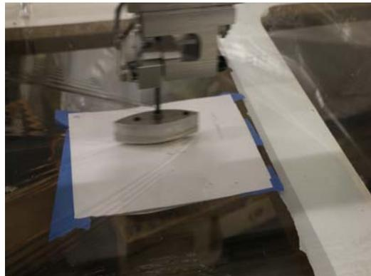
**Figure 4** Flow around a diamond airfoil (wedge angle  $15^\circ$ ) (see online version for colours)
