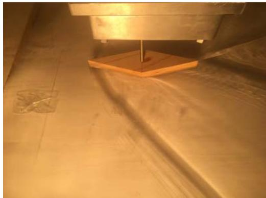
**Figure 5** A picture of the Busemann's biplane with the hydraulic analogy (see online version for colours)
