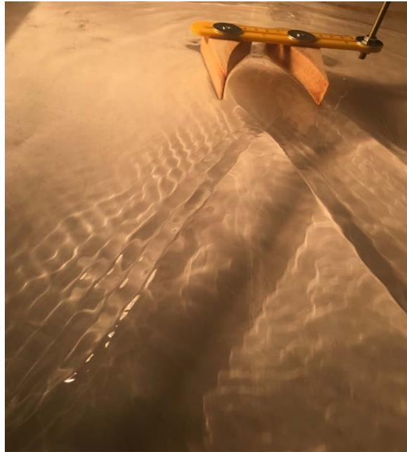
**Figure 12** A simple arrangements to demonstrate shallow water surface waves (see online version for colours)
