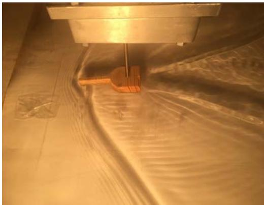
**Figure 10** Shock formations inside the convergent/divergent nozzle (see online version for colours)
