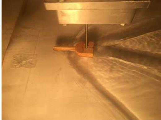
**Figure 9** Shock pattern for flow around a cylinder with a spike (not so sharp) (see online version for colours)
