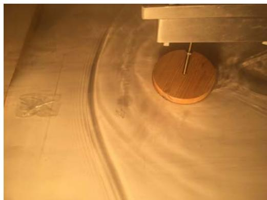
**Figure 8** Flow over a cylinder with a sharp spike (see online version for colours)
