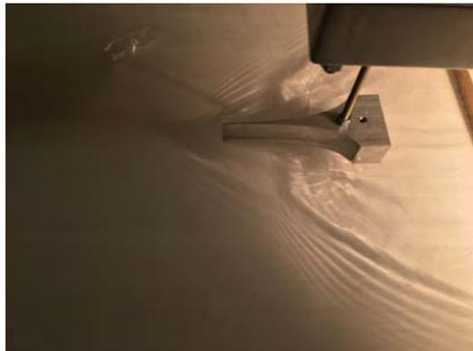
**Figure 7** A bow shock is formed in front of a moving cylinder (see online version for colours)
