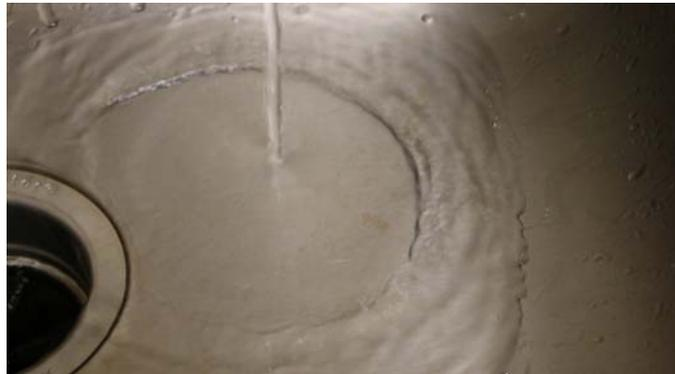
In Figure 13, the flow pattern around a diamond airfoil, using this simple arrangement, is shown. Notice both compression and expansion waves. Controlling the speed of the water stream and the height of the water layer allows the variation of the Froude number.
