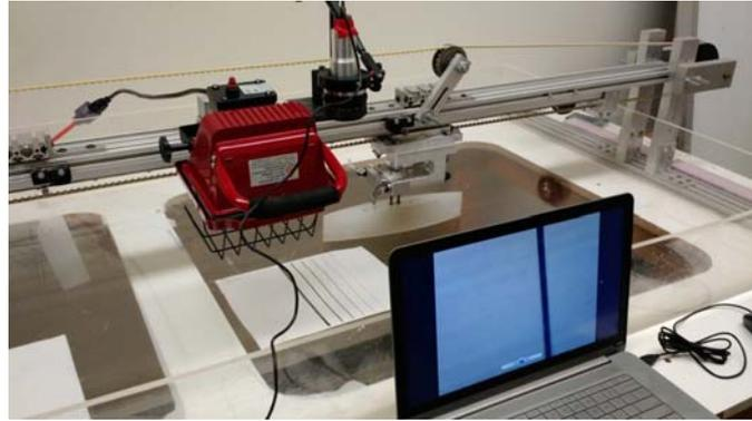
**Figure 15** Wave measurement
