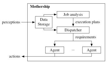
The general structure of the framework is shown in Figure 1. The user configures the application via a command-line interface, which in turn calls the session manager, to handle the necessary state of a connection with MASSim over multiple simulations. The session manager relies on the message subsystem to communicate with MASSim over a TCP/IP socket. It instantiates a Mothership for each simulation and transfers the perceptions and actions between the Mothership and the message layer.
