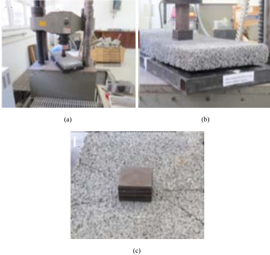
Figure 6 Bending tests on pervious concrete slabs (see online version for colours)
