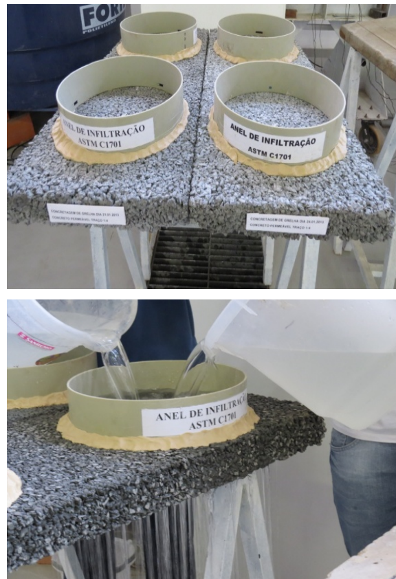
Figure 8 Procedure for testing the water infiltration rate (see online version for colours)
