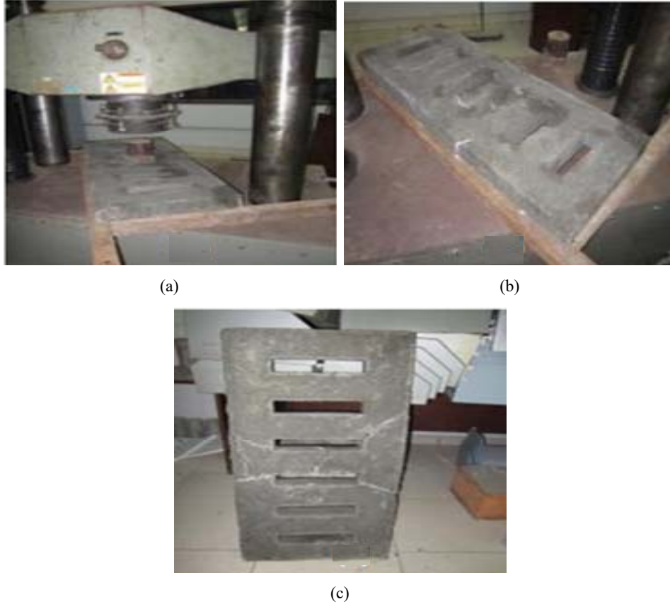
Figure 7 Bending test on conventional concrete grid from DEP (see online version for colours)
