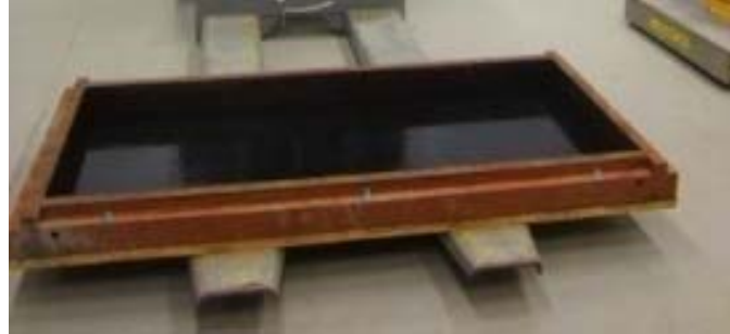
Figure 1 Cedar wood mould used to for the pervious concrete grids (see online version for colours)
