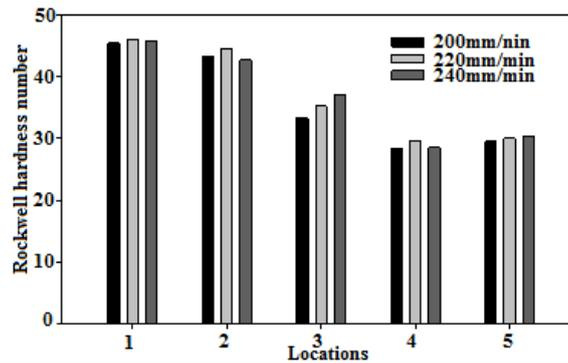
Higher heat input associated with weld speed leads to increase in hardness at HAZ. However as the laser beam heat affects the Al side, Al gets softened due to its low melting point and hardness is considerably reduced even at the base metal zone.
