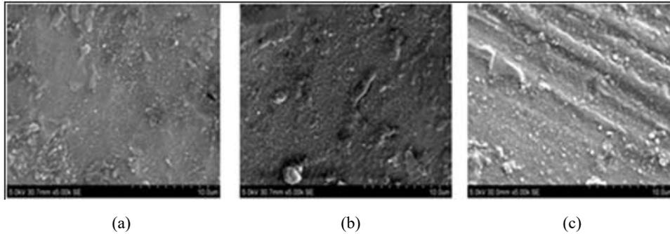
Figure 7(a), Figure 7(b) and Figure 7(c) show fine grain structures at the speed of 240 mm/min. it is noted that grain size decreases with increase in speed. Comparing with weld speed 200 mm/min, at 240 mm/min grain structures are uniformly distributed and are smooth in texture. Thus, higher welding lead to grain refinement both in fusion and HAZs.
