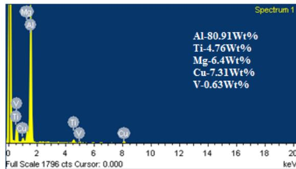
Spectrum analysis indicates that Al content is enhanced to 80.91% whereas Ti content is reduced to 4.76% and results further increase in hardness at 240 mm/min. It is observed that reduction in Ti is not affecting the increasing trend of hardness, as 0.01% Ti is enhanced to 4.76% in Al alloy. This finding is also supported by the higher hardness distribution at fusion zone viewed from the Al side as per Figure 5. Hence, higher welding speed improves the strength of dissimilar weld joints.
