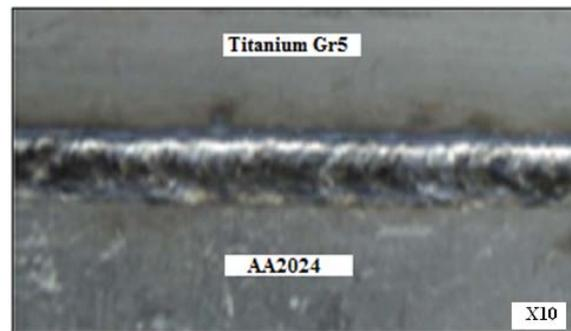
As the welding speed increases, crack formation tendency gets eliminated in Ti/Al joints. Also, clean surface morphology is noted at higher welding speeds.
