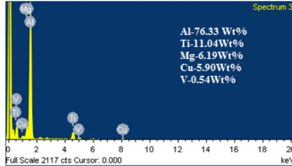
It is seen that welding speed is an important factor on heat flow in welding. These, in turn, affect the metal penetration depth, shape and final solidification structure of the fusion zone. Both shape and microstructure of the fusion zone are influencing considerably the properties at the weldment. The sample at the speed of 240 mm/min formed at the fusion zone is observed by EDS and is shown in Figure 9.
