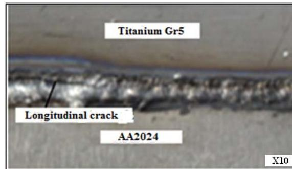
**Figure 3** Surface morphology at speed 240 mm/min (see online version for colours)
