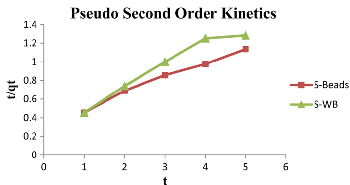
Figure 6 Pseudo second order plot for the adsorption of Cr(VI) on Saraca indica beads (see online version for colours)
