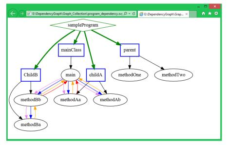
At least two forms are presented for representation of one graph. Here we have presented only text, matrix and graph view of class hierarchy relationships as example. Figure 9 shows sample text view and matrix view form of DA-OOP. Figure 10(a) shows text view and 10(b) shows matrix view of CHG of DA-OOP separately. Figure 11 presents the graph view of dependency graph which is shown in browser using Graph-Viz tool.
