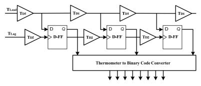
However, the Vernier delay line architecture has two main drawbacks. Namely, the calibration required to precisely control the resolution in a predictable way. The other problem shows up for a large input range or very fine resolution. In this case, an excessive number of delay stages are needed, which lead to an area penalty and stringent mismatch requirements.
