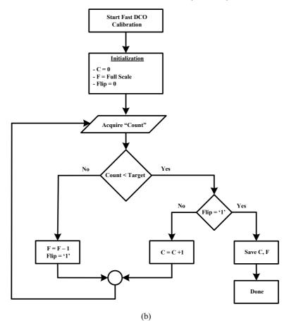
Figure 10 (a) Configuration used for the calibration of the fast DCO (b) determining the coarse and fine control codes for the fast DCO flowchart (continued)
