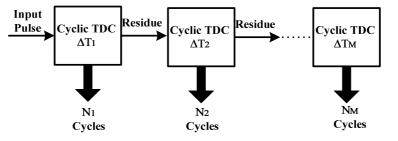
As a result of this architecture, the relationship between the measurement time and the input pulse width is no longer a linear relation as it was in the normal cyclic TDC, as shown in Figure 5. Thus, the throughput of the system is less dependent on it resolution.
