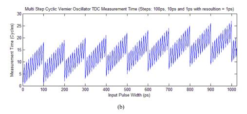
*Practical implementation considerations:* Figure 6(a) shows the waveforms both oscillators of a conventional cyclic TDC. The residual time of a given measurement is simply the time difference between the two edges before phase flipping. Thus, for the multi-step cyclic TDC, the oscillators need to be re-enabled using the edges of the residue for every new time step. In this way, the multi-step cyclic TDC architecture can be implemented using the same hardware of a single TDC stage.
