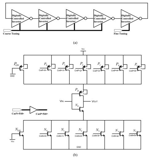
Figure 8 (a) Coarse and fine tuning for the DCO (b) inverter cell used in the implementation
