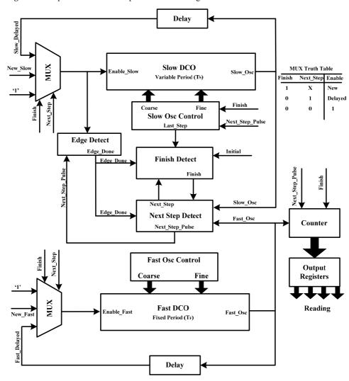
At the start of a new measurement, the edges of the signal to be measured are fed to the enable terminals of the digitally controlled oscillators (DCOs). When the lagging edge enables the fast DCO, the 'Edge\_Done' signal is asserted which resets the 'Finish' signal. During a given time step ( $\Delta T$ ), the oscillations of the DCOs are sustained by feeding a high logic value to their enable terminals.
