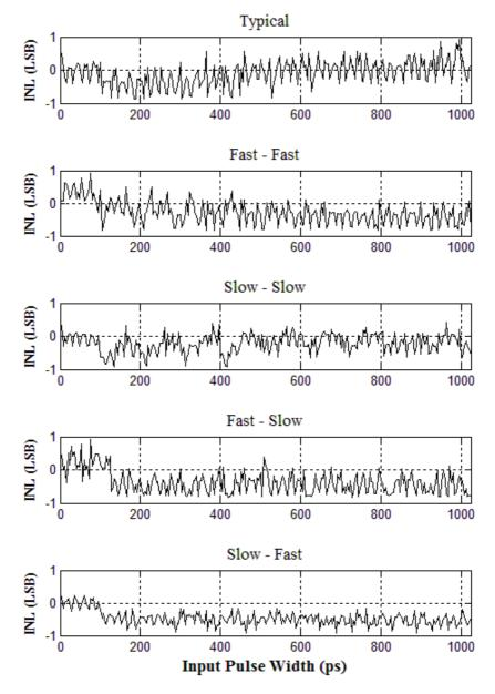
Figure 14 INL of the TDC when programmed for time steps of: 100 ps, 10 ps and 4 ps and an input range of 1,024ps at different process corners
