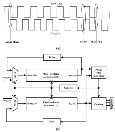
Figure 6 (a) Waveforms of the oscillations and the measurement residue, (b) simplified block diagram of the proposed multi-step cyclic TDC
