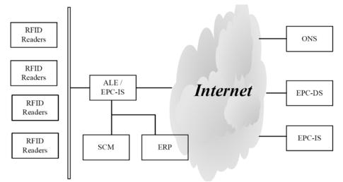
Figure 4 Basic communication model of mobile RFID
