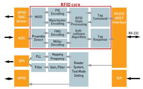
Figure 12 Block diagram of the UHF band mobile RFID reader (see online version for colours)
