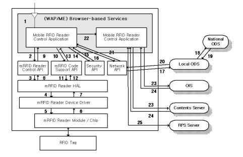
Figure 15 Scenario of secure mobile RFID M/W terminal function
