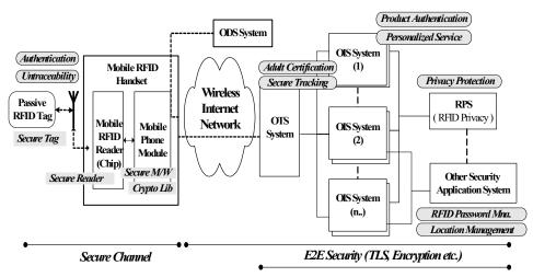
The main functions of the proposed service model are the provision of WIPI-based mobile security middleware, tag authentication, tag tracking prevention, reader authentication, message security, non-traceable payment and policy-based privacy protection (Ohkubo et al., 2003; Mobile RFID Forum of Korea, 2005a; Park, 2008).
