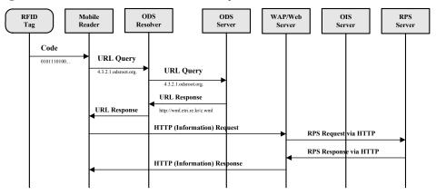
Figure 8 Detailed mobile RFID's code resolution process
