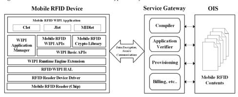
Figure 21 Service structure of mobile RFID crypto library
