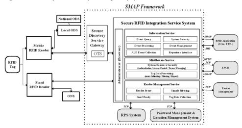
Figure 17 Arch. of portal discovery service gateway system
