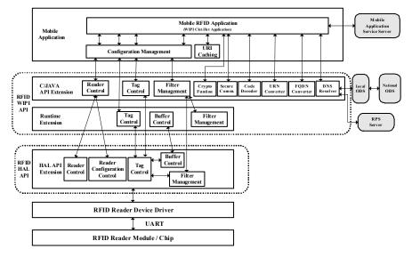
Figure 13 Function block diagram of mobile RFID middleware platform in the mobile phone
