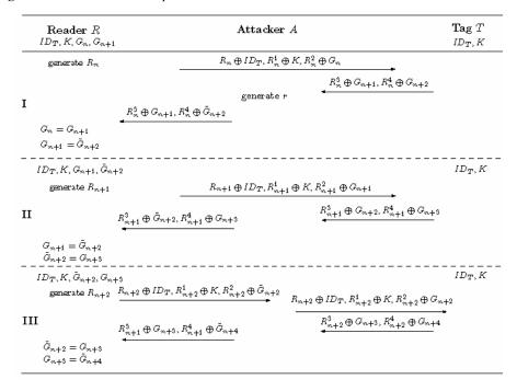
Figure 3 Attack on the basic protocol
