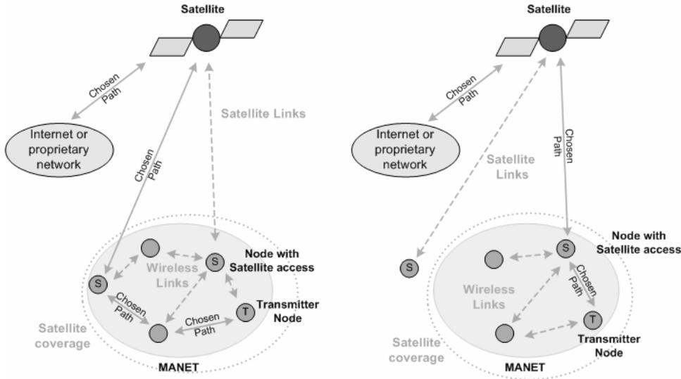
**Figure 6** Hybrid MANET-satellite challenge: satellite as relay between two MANETs
