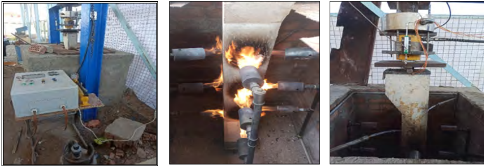
Figure 4 Specimens subjected to fire exposure under pre-loading curve (see online version for colours)
