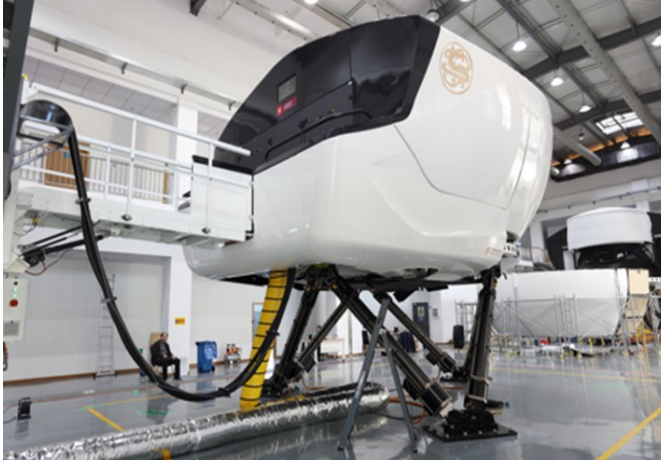
Figure 1 Stewart flight simulator motion platform (see online version for colours)
