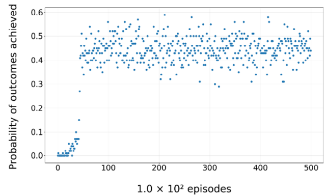
Figure 6 Probability of generating feasible master production scheduling results averaged over every 100 episodes during the training process (see online version for colours)
