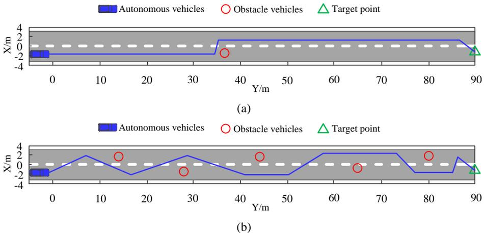
**Figure 6** Obstacle avoidance path selection results of Zhang and Zhang (2022) method: (a) single obstacle and (b) multiple obstacles (see online version for colours)
