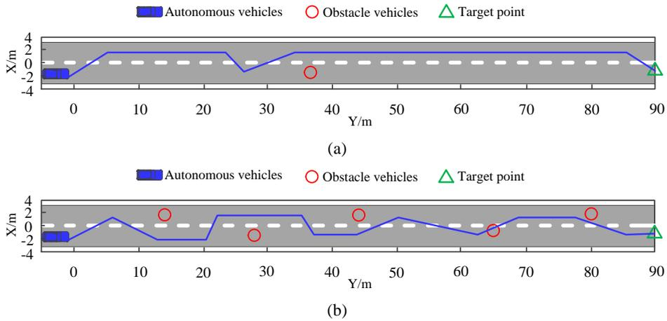
**Figure 7** The obstacle avoidance path selection results of the proposed method: (a) single obstacle and (b) multiple obstacles (see online version for colours)
