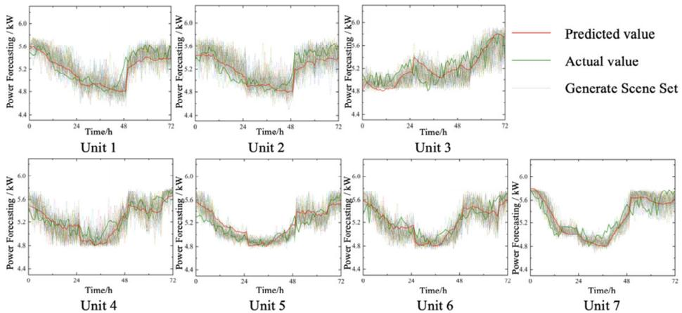
From the figure, it can be observed that the scenario set generated by SLEP effectively covers the variation range of actual wind power while exhibiting a reasonable distribution pattern that reflects the possible fluctuations of wind power at different time steps. This
