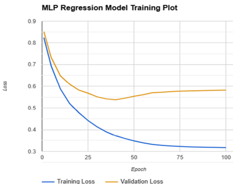
Figure 7 Plot showing the training and validation loss curves of an MLP regression model over 100 epochs (see online version for colours)
