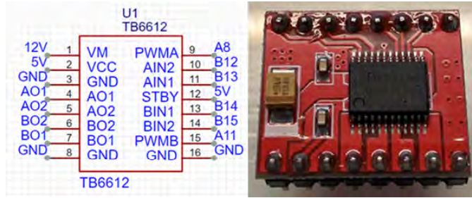
Figure 10 TB6612FNG motor drive module (see online version for colours)
