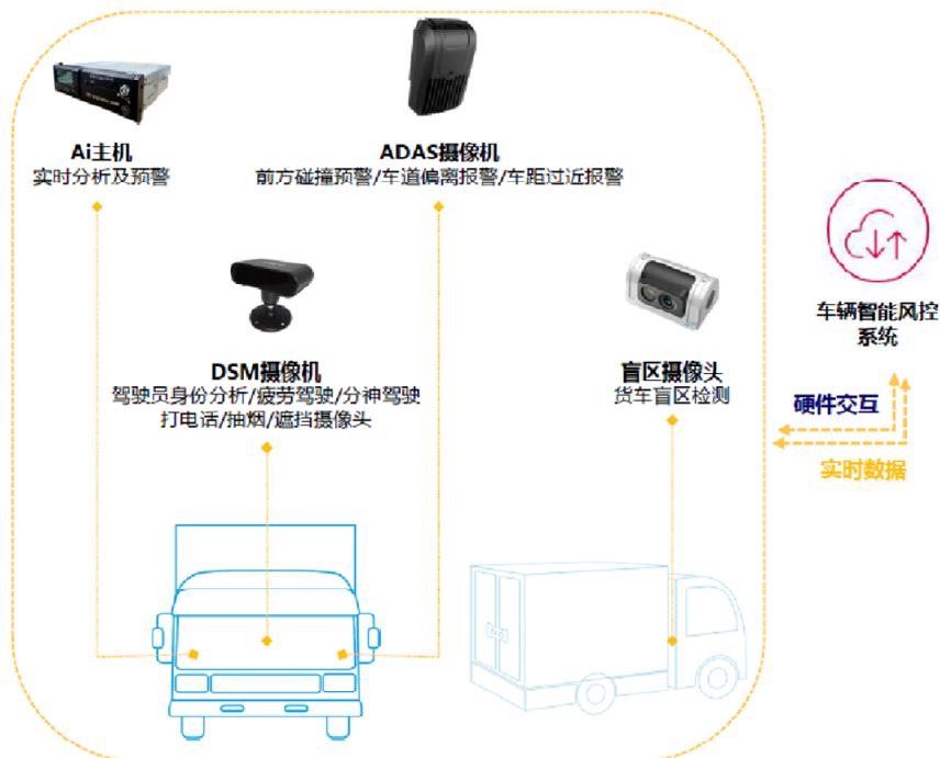
Figure 2 The hardware of the integrated AI system (see online version for colours)
