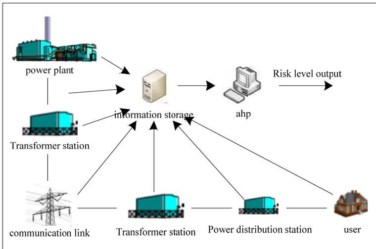
The power communication network risk assessment was conducted by the experimental power grid company using the scenario depicted in Figure 1. Table 1 enumerates the precise dimensions and pertinent parameters of this experimental power grid company.
