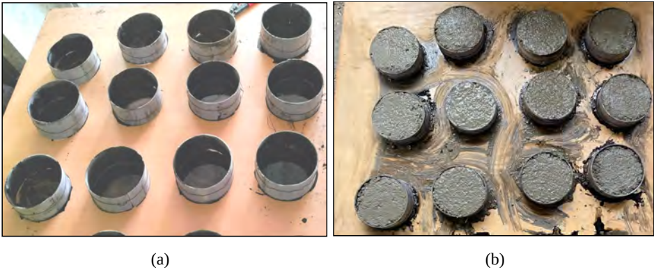
Figure 2 Mould preparations (a) before casting (b) cast specimens (see online version for colours)
