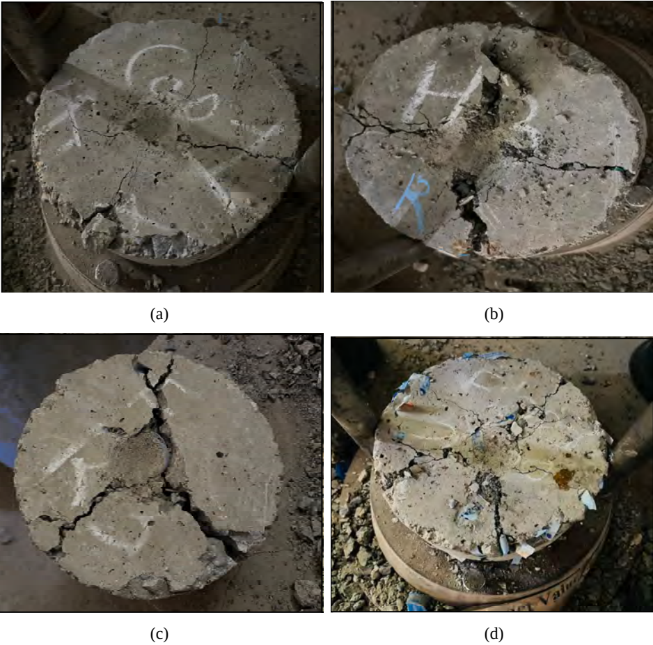
Figure 6 Crack pattern for tested disc specimens for (a) fibres (b) cap (c) cap rings (d) labels (see online version for colours)
