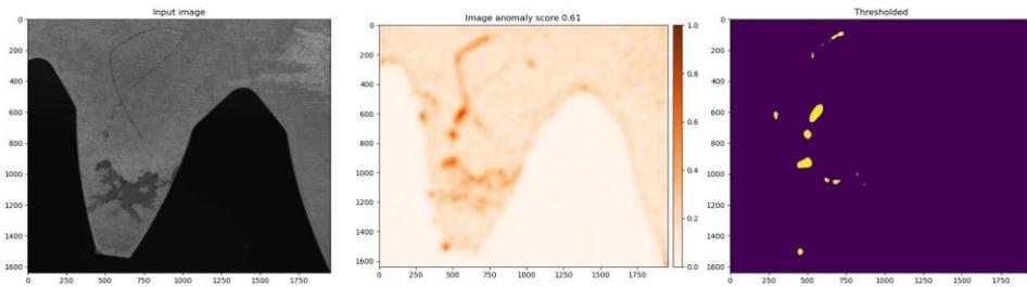
**Figure 17** Example from the industry manufacturing dataset with classification. Front view. Image anomaly score 0.73. True positive since there is wear on the power skiving tool from industry machine usage over time (see online version for colours)
