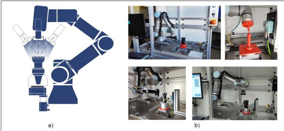
Initially, a portal axis system was pursued due to its high accuracy. However, due to ongoing delivery delays, a less accurate and more flexible system was used instead. This system features a lightweight articulated robot (UR 5e, Universal Robots) that is significantly more flexible and will allow for investigations to be extended to other tool geometries in the future.
