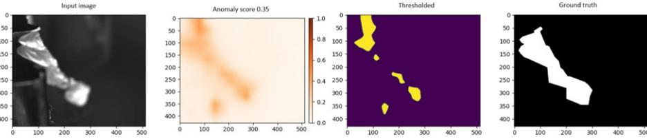
**Figure 19** Example from the industry manufacturing dataset with segmentation and ground truth. Side view. Image anomaly score 0.35. True positive since there is a breakout (see online version for colours)
