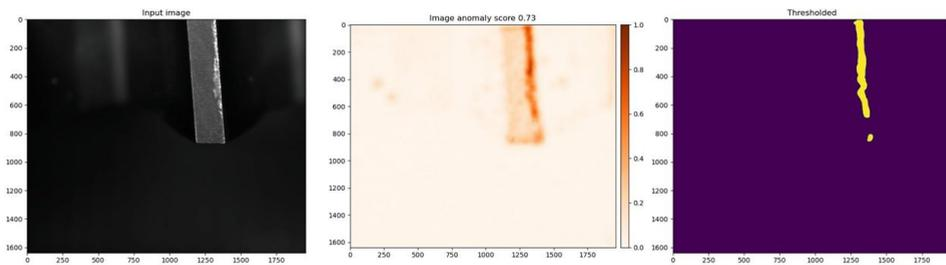
**Figure 18** Example from the industry manufacturing dataset with segmentation and ground truth. Side view. Image anomaly score 0.35. True positive since there is a breakout (see online version for colours)
