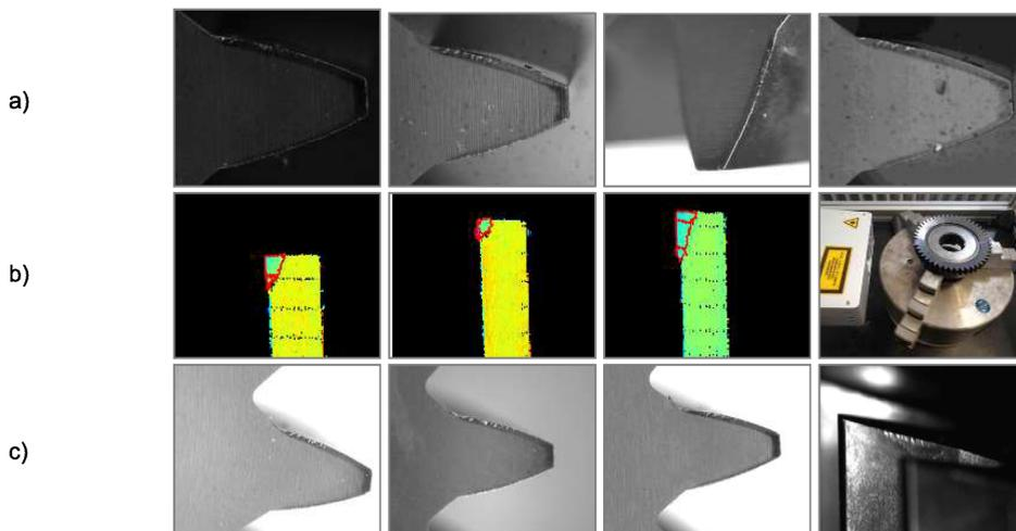
A decision was made in favour of a variant with simple incident lighting using a ring light (see Figure 5(c)). The camera system comprises a monochrome 5-megapixel Basler acA2040-35gm camera (with a sensor size of 2/3 inch and a 1/1.8 inch Sony IMX265, manufactured by Basler AG), a macro lens Opto 100-MC100 (with a working distance of 87 mm, aperture of 14, depth of field of 0.4 mm and a field of view of  $8.8 \times 6.6 \text{ mm}$ ,
