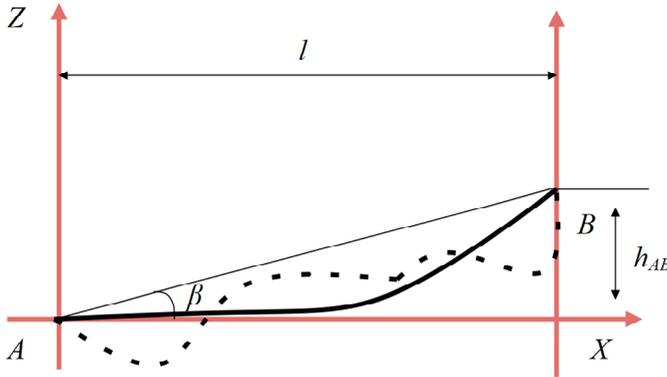
**Figure 2** Galloping conductor, (a) vertical vibration of galloping conductors (b) horizontal vibration of galloping conductors (see online version for colours)
