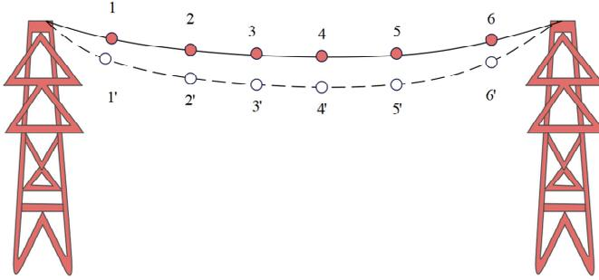
We assume that  $N_t$  tags are installed along the wire, and the coordinates of each tag  $l_i$  are expressed as  $(x_i, y_i, z_i)$ , where  $i \in [1, N_t]$ . In time  $T$ , if the position information of the tag on the wire is measured at time intervals  $\Delta t$ ,  $N_t \times N_t$  measured values can be obtained, where  $N_t = \frac{T}{\Delta t}$ . When the measured values are expressed by matrix  $L$ , the following results are obtained (Khan et al., 2023):
