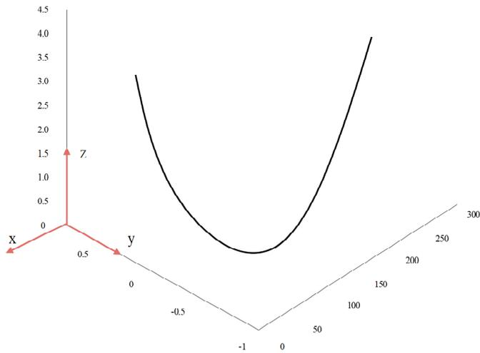
In order to use the principle of compressed sensing, we regard the wire as a curve in Cartesian coordinate system. Under this model, whether the wire is galloping or stationary, the wire can find its corresponding curve in the coordinate system, and every
