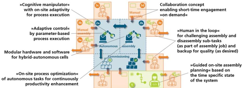
The matrix production concepts outlined in the prior art typically provide a central or cloud-based planning level in which all tasks in a process chain are decomposed into subtasks, including transfer operations and the assignment to specific assembly cells. This also includes resource planning, both on the plant side in terms of necessary skills, necessary tools and available capacities, as well as the requirement for components.
