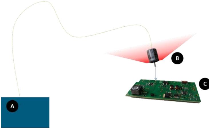
For in-process optimisation of the overall plugging time, the initial speed of the robot along the path between A and B is slow so to plug all capacitors safely. Based on this initial condition, the robot’s speed along the path is increased step by step to optimize plugging times. As the speed increases, the number of out-of-tolerance approaches at position B increases until the overall time over many plugging processes increases again due to a high proportion of “failure plugging’s”.
