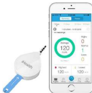
Figure 3 A glucometer add-on for mobile phones (see online version for colours)
