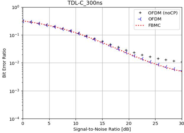
**Figure 11** Bit error rate using PHYDYAS filter in TDL – C
