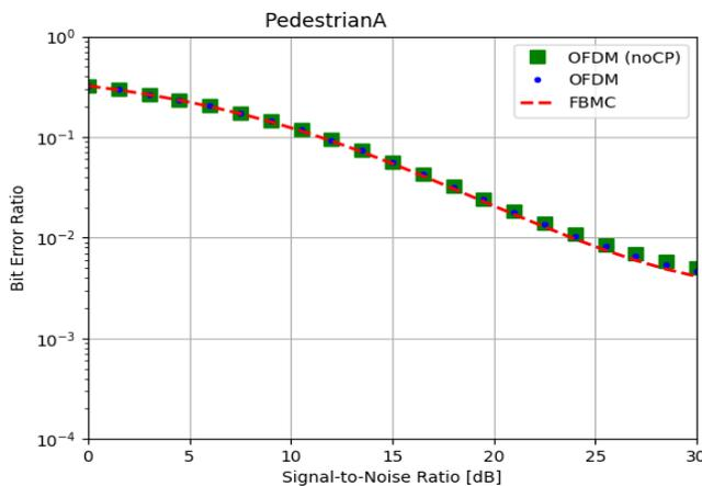
**Figure 15** Bit error rate using PHYDYAS filter in vehicular channel
