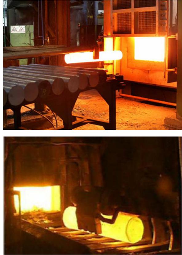
The reference of the automatic positioning system represents the displacement of the billet relative to the rail axis, while the output of the system is represented by the position of the unloading arm. The set point of the system is given by a billet detection system which is based on a video camera and determines the displacement of the billets relative to the roller way axis in mm.
