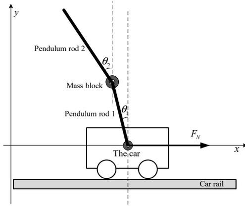
The total kinetic energy and total potential energy of the double inverted pendulum are expressed as follows:
