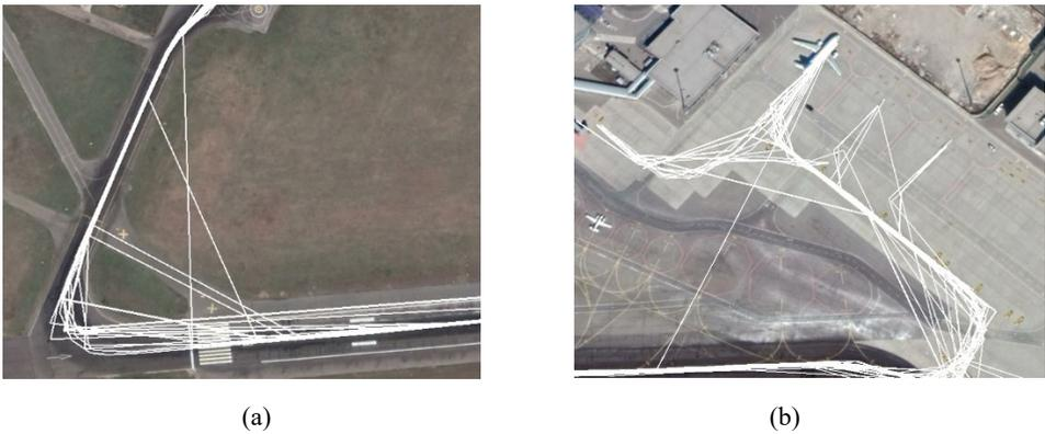
**Figure 5** Location of additional receivers A1-A3 (a) and track (yellow) correspondence to runway and taxiways geometry (A2) (b) (see online version for colours)
