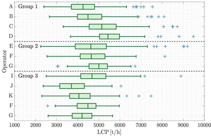
**Figure 6** A comparison of means using the Tukey-Kramer method showing the 95% confidence on estimates of the mean LCP for different operators.
