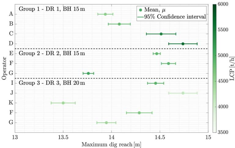
Note: The confidence intervals are obtained using the Tukey-Kramer method and represent the 95% confidence interval of the mean maximum dig reach.
