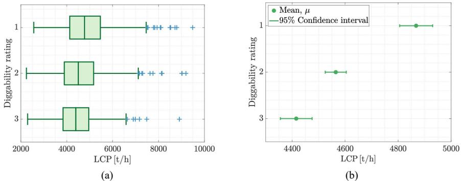
Notes: The condition with the lowest rating of 1 has the highest mean LCP of 4,868 t/h while the highest, 3, has the lowest LCP of 4,415 t/h.
