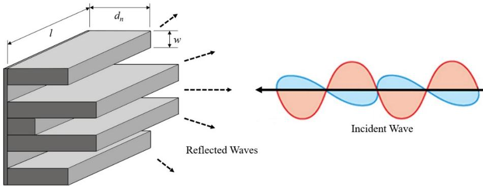
In this paper, considering the frequency to be analysed, two single-band diffusers which are applied to the frequency ranges of 2 to 3 GHz and 4 to 5 GHz respectively and a dual-band diffuser combined with two single-band diffusers were designed. In Schroeder's 1D QRD, the width of a well ( $w$ ) is determined by  $\lambda_{\max}$  and the depth of well ( $d_n$ ) is determined by  $\lambda_{\min}$  as equations (1) and (2).
