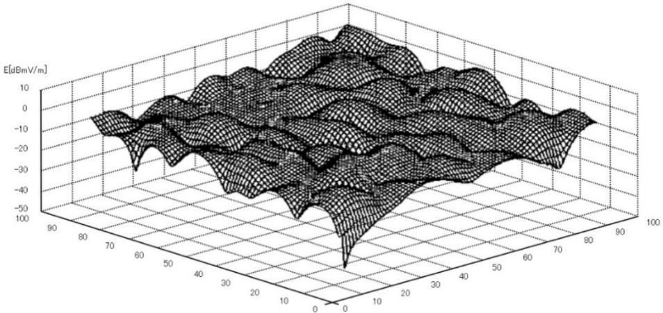
To investigate the polarisation characteristics when a diffuser is attached in the reverberation chamber, the values of  $E_x$ ,  $E_y$  and  $E_z$  for 34,246 cells of the x-z plane ( $y = 151$  cross-section) are extracted and the cumulative distribution function was found for 75% of samples. The overall distribution followed a chi-square distribution.
