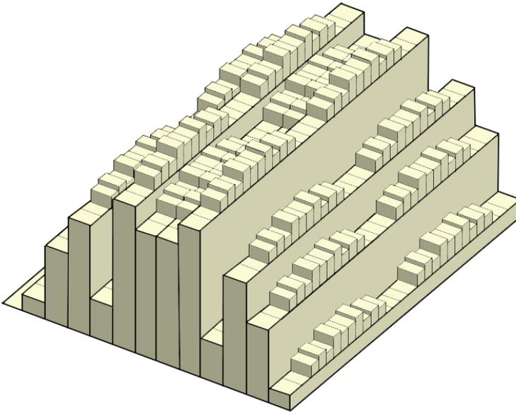
As the length ( $l$ ) and period of QRD increase, the efficiency of the reverberation chamber is improved. In this paper, considering the size of the reverberation chamber, two single-band stirrers (QRD#1 and QRD#2) in Figures 4 and 5 are designed to be one period diffuser. The dual-band diffuser in Figure 6 is designed by combining one period QRD#1 and two periods QRD#2. When electromagnetic waves of 2 GHz are scattered,
