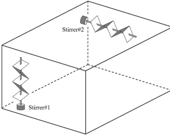
**Figure 2** Suggested reverberation chamber with a diffuser
