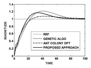
Figure 5 Time domain output for step input of Sys. 4: G A, A C O, GA-ACO
