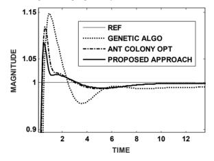
Figure 6 Time domain output for step input of Sys. 5: G A, A C O, GA-ACO
