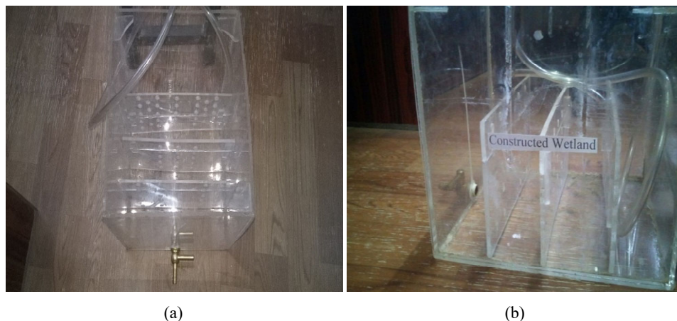
Figure 4 (a) Top and (b) side views of constructed wetland (see online version for colours)
