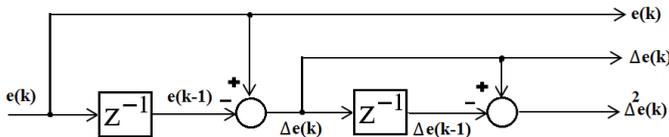
The principle structure of fuzzy PID controller is shown in Figure 3.  $\Delta u(k)$ ,  $\Delta u_s(k)$  and  $S_{\Delta u}$  are the incremental controller output, scaled version of incremental controller output and the output scaling factor, respectively.
