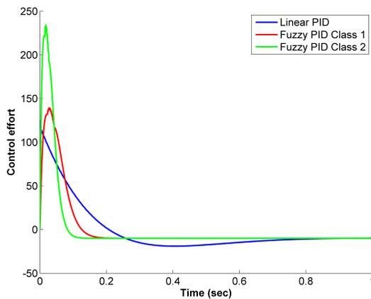
The output step responses of the nonlinear plant and the control efforts of linear and fuzzy PID controllers are shown in Figures 10 and 11. Sampling time  $T_s = 1$  ms is considered for simulation. The time-domain performance data related to the linear and
