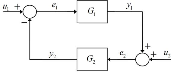
*Proof:* Consider a closed loop control system as shown in Figure 9. The following equations govern the closed loop system.
