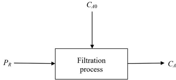
**Figure 3** Black-box model structure of filtration process
