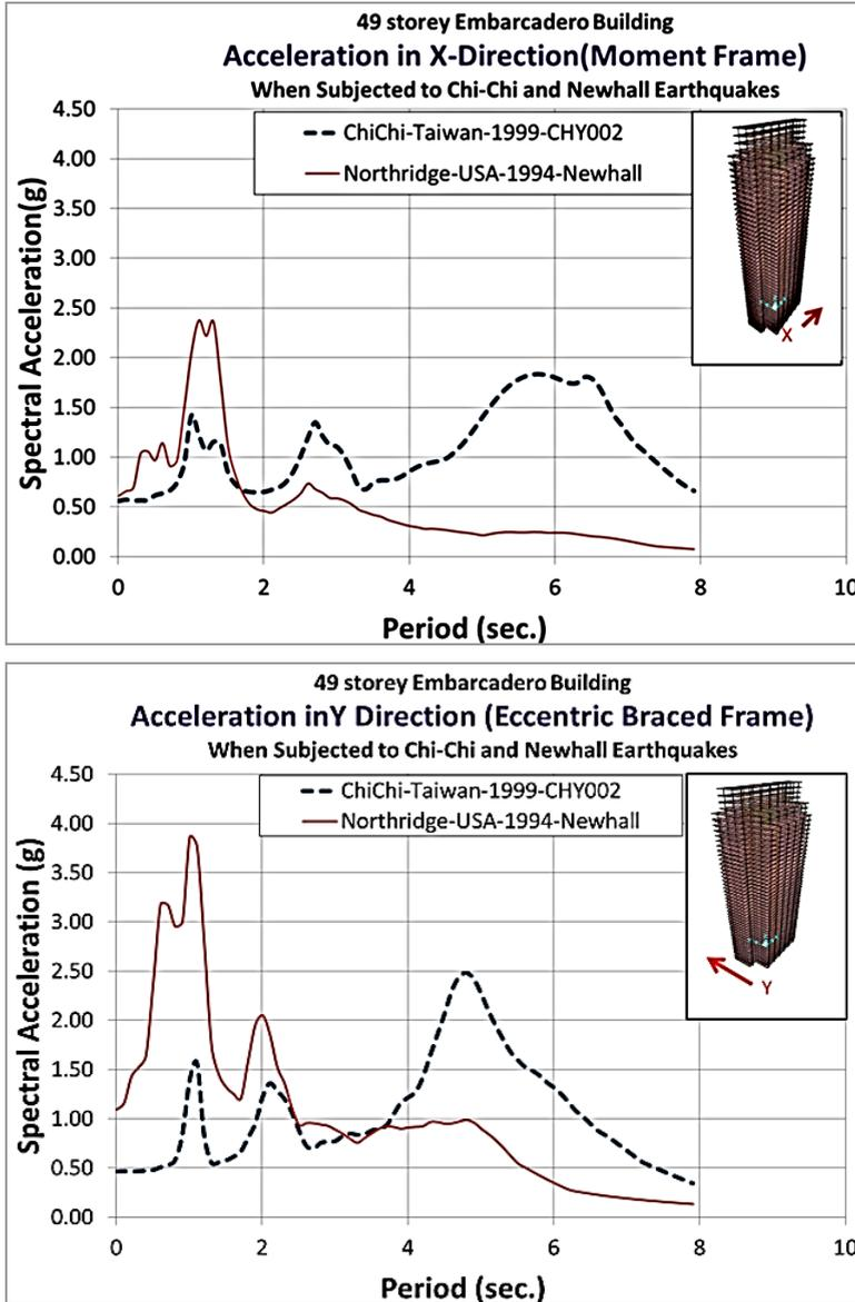
In the moment frame direction, the Northridge-Newhall produced a relatively low peak base shear of 0.03 W; however, ChiChi-002 ground motion generated a peak base shear of 0.15 W, which is five times that of the Northridge-Newhall-generated base shear. Apart from higher peak values, the ChiChi-002 also generated a higher number of large amplitude cycles of base shear in both directions. The higher number of large amplitude
