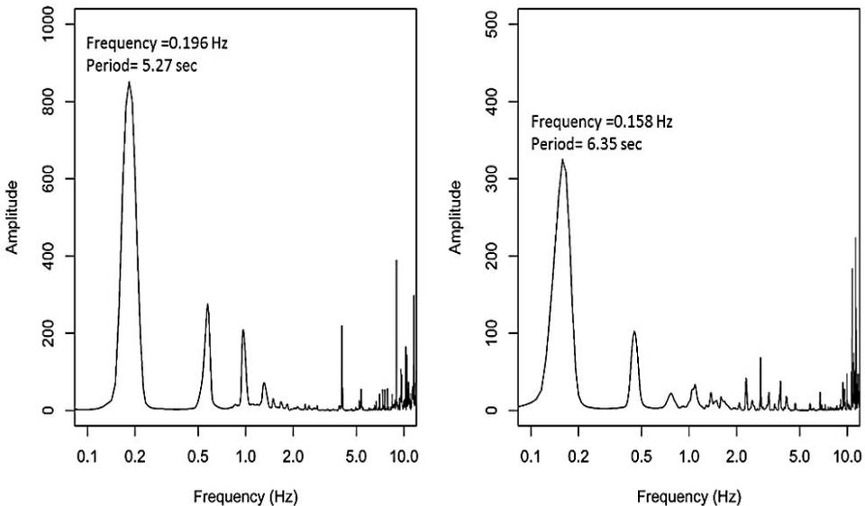
**Figure 9** Roof displacement response of model and structures (see online version for colours)
