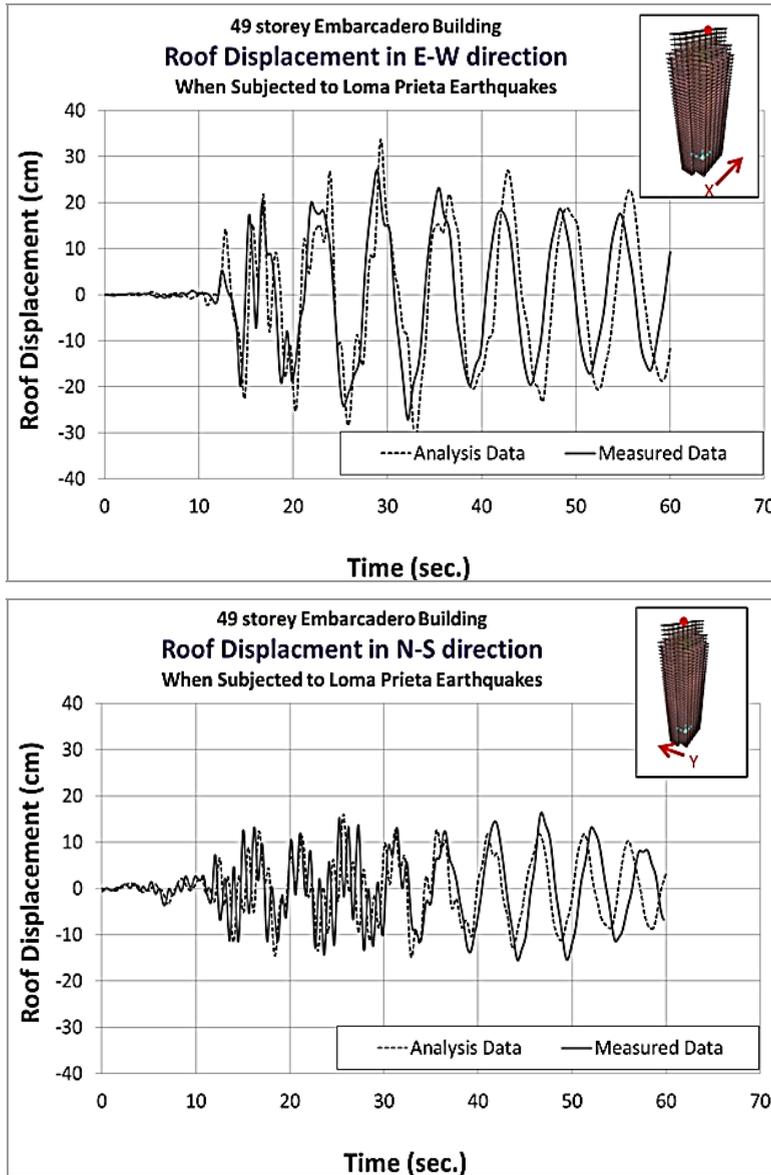
Displacement response of measured data and analysis data also show a good correlation. The plot of the displacement time history in Figure 9 at the 44th floor for measured response compared to the model shows that the response of the moment frame (E-W) is initially very sensitive to the ground shaking. The peaks predicted by the model exceed slightly the measured peaks. Measured data show that peak displacement in E-W
