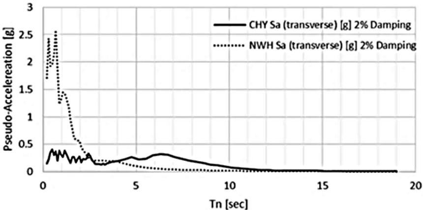
**Figure 7** Pseudo-displacement spectra of the far-field and near-field (dashed line) ground motions used in the study (see online version for colours)
