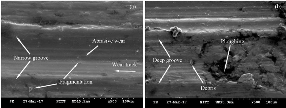
**Figure 13** EDS analysis (a) low wear loss and (b) higher wear loss specimen (see online version for colours)
