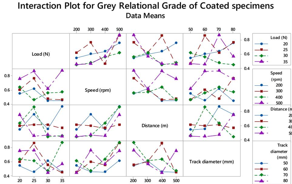
From the interaction plot shown in Figure 9 for coated specimens, interaction effects between speed and other input parameters are significant and also between load and track diameter. In between other parameters a moderate relationship exists.
