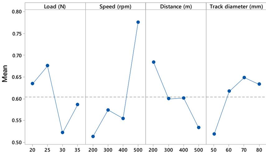
**Figure 8** Interaction plot for grey relational grade of uncoated specimens (see online version for colours)
