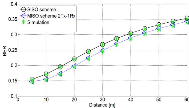
Figure 5 depicts both SISO scheme and MISO (2Tx1Rx) scheme in absence of interference. It can be seen that as expected the BER performance is enhanced by increasing the number of transmitted antennas.
