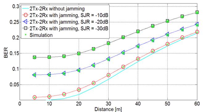
Figure 9 depicts the BER performance of the 2Tx2Rx MB-OFDM UWB MIMO scheme in presence of interference for different SIR values (-10 dB, -20 dB and -30 dB). It can be seen that increasing the number of transmitting and receiving antennas improve the transmission range of the MB-OFDM UWB communication systems. Yet, the presence of high inband interference signal such as the IEEE802.11n WLAN operating services may cause a harmful effect on the performance of the UWB systems.
