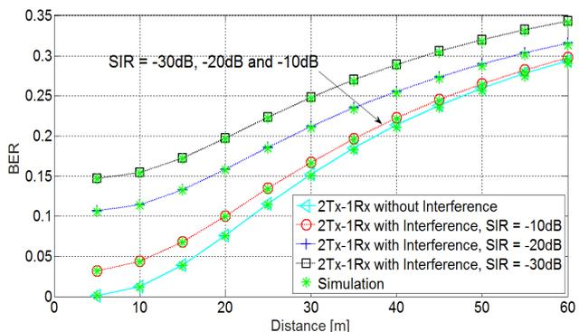
Figure 7 depicts the impact of presence of the IEEE802.11n interference at different SIR values on the considered scheme. It can be seen that the BER performance of the MISO (2Tx1Rx) scheme is severely deteriorated due to presence of high power in band interference.
