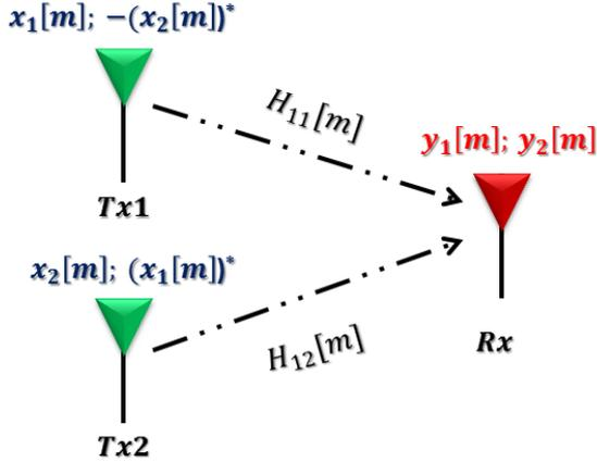
At block time  $i$ , the symbols  $x_1[m]$  and  $x_2[m]$  are transmitted by the first and second transmit antennas, respectively; at block time  $i + 1$ , the symbols  $-(x_2[m])^*$  and  $(x_1[m])^*$  are transmitted by the first and second transmit antennas, respectively. Consequently, the received data from two consecutive blocks are
