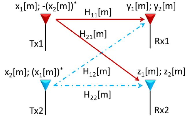
In the receiver side both  $x_1[m]$  and  $x_2[m]$  can be estimated as (Foerster, 2003):
