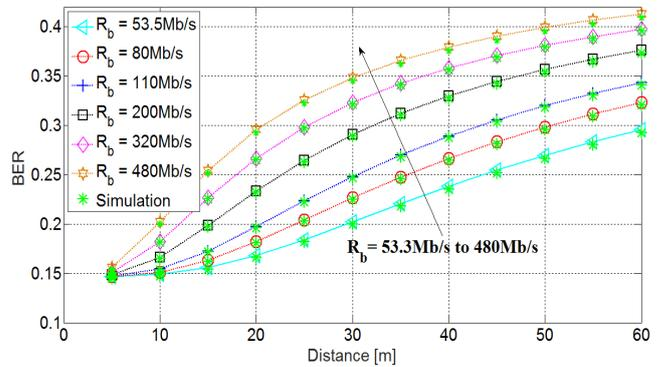
Figure 8 depicts the impact of varying the data rate of the 2Tx1Rx MB-OFDM-UWB system from 53.3 Mb/s to 480 Mb/s in presence of the IEEE802.11n interference at  $SIR = -30dB$ . It can be seen that increasing the data rate in presence of high power inband interference signal will degrade the quality of service of the desired system at certain coverage distance. From all the previous figures it also can be seen that the simulation results are in a good match with the derived theoretical results.
