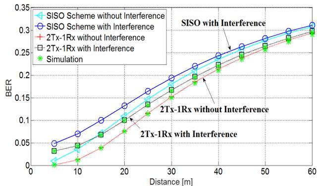
Figure 6 depicts the impact of presence of the IEEE802.11n interference on the BER performance of both the SISO and MISO (2Tx1Rx) schemes. It can be seen that at  $BER = 0.05$ , a degradation in the MB-OFDM UWB coverage distance could reach up to 5 m at  $SIR = -10dB$ .
