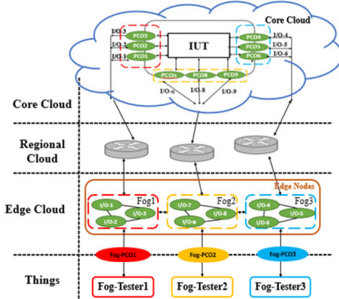
Figure 4 Distributed cloud testing architecture (see online version for colours)
