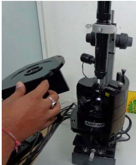
Figure 2 R_a measurement of FG-260I by AFM (see online version for colours)
