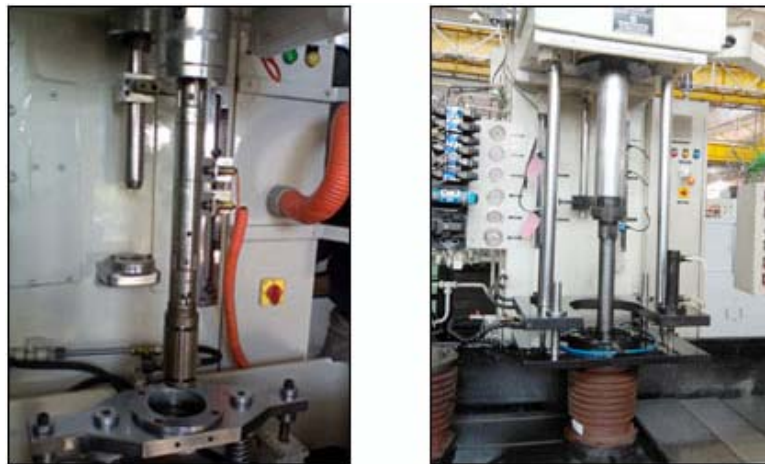
Figure 1 Honing head with tooling (see online version for colours)
