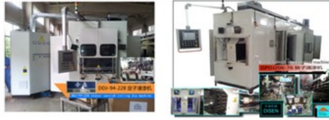
Stator varnish rolling dip machine, Rotor varnish trickling machine
