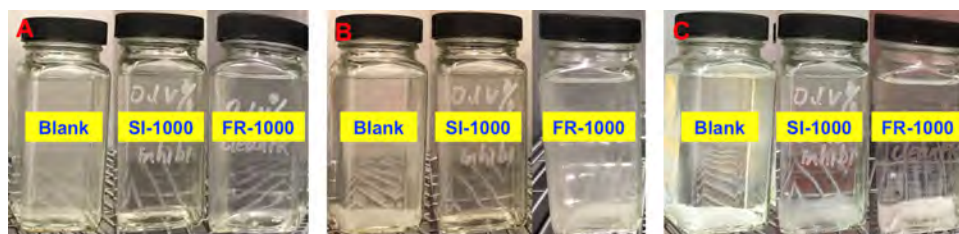
Figure 8 Scales formed when two water samples mixed together (bulk solution A and bulk solution B; SI or FR-2 was mixed with bulk solution B first before mixing with A), the mixtures were heated at 120°F (49°C) for different periods of time, (a) 0 min, (b) 20 min and (c) 20 hours (see online version for colours)
