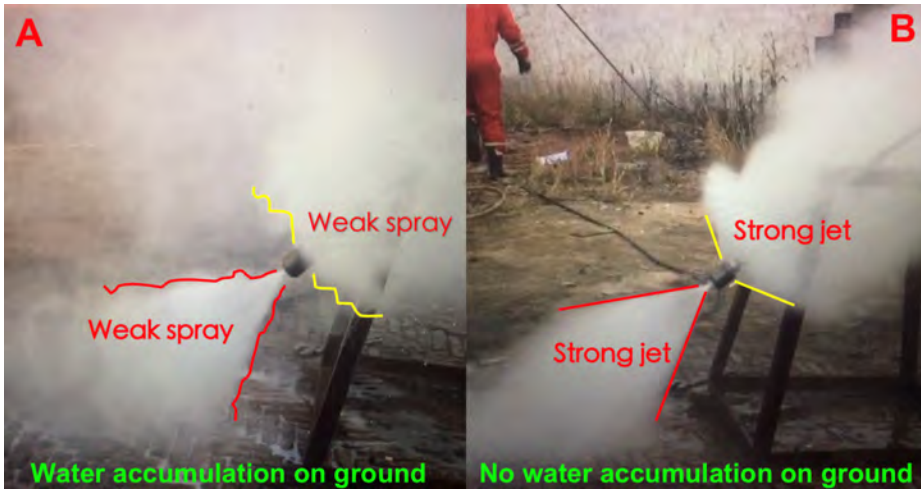
Figure 6 Water spray through coiled tubing with a rotary nozzle, (a) water only (b) water with FR-2 at 1,000 ppm (see online version for colours)
