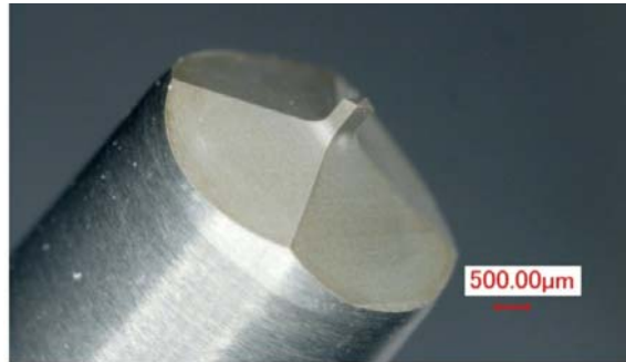
Figure 12 Fabricated tailored micro end mill with optimum design parameters (see online version for colours)
