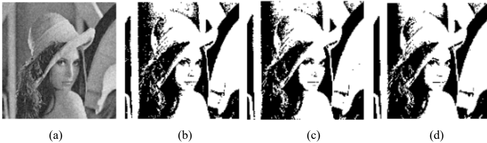
Figure 5 Segmentation result of adding Gaussian noise, (a) source image plus Gaussian noise (b) rapid 2-otsu segmentation results (c) 3-Otsu segmentation results. (d) segmentation results of the proposed algorithm
