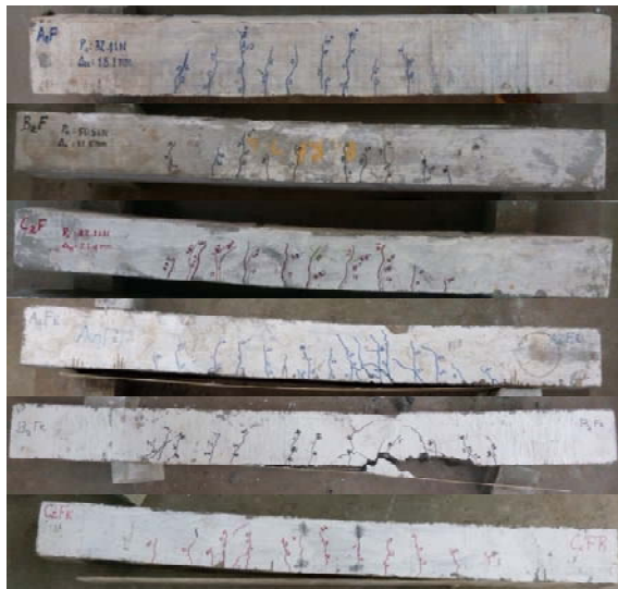
Figure 10 Crack pattern at collapse for the tested beams (see online version for colours)
