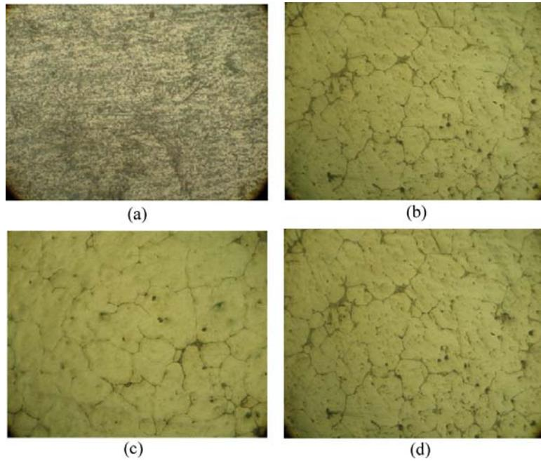
**Figure 13** (a)  $C_1$  – Al 6061 alloy after wear; (b)  $C_2$  – reinforced composite after wear and (c)  $C_3$ ,  $C_4$  and  $C_5$  – reinforced composites after wear
