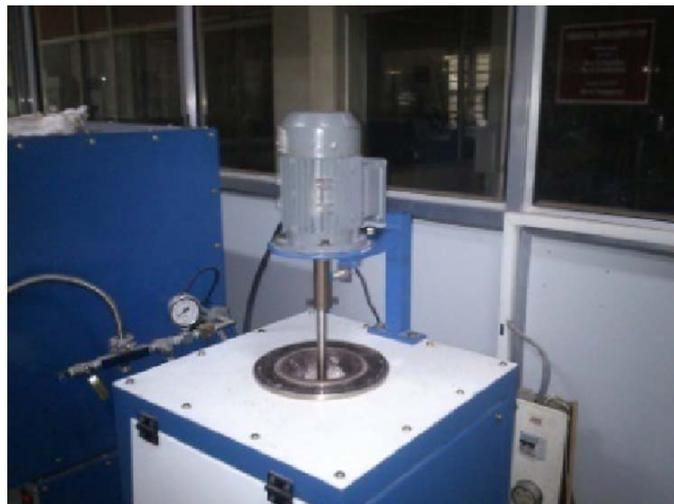
**Figure 4** Casting of composite (see online version for colours)
