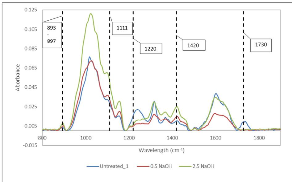
In the present study the peak around 1,220  $\text{cm}^{-1}$  is also lower for the alkaline treated fibres, showing that lignin component has also been partially removed. Since hemicellulose and lignin (partially) have been removed from the natural fibre after the alkaline treatment, the treated fibre has a higher ratio of cellulose present in the fibre.
