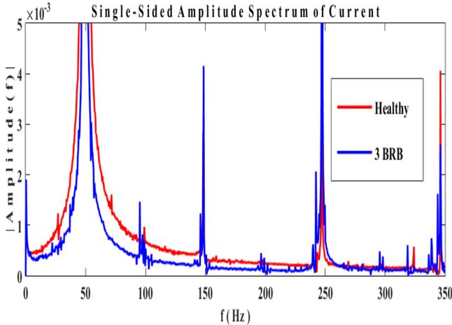
FFT was then performed on the current signals and analysis performed in the frequency domain. Figure 8 shows a comparison between the amplitude of power spectra of the current of a healthy motor and that of motors with the studied BRB faults under the same load conditions.
