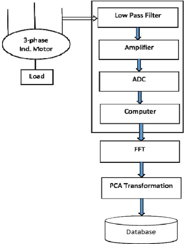
Figure 2 Flowchart for the proposed ‘scheme 1’ (see online version for colours)
