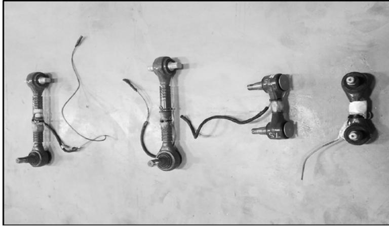
Prior to installing the rods on the bus, they were calibrated for force in a bench test (with a hydraulic actuator and a load cell). Figure 6 presents the obtained calibration curves for each of the link rods, which correlates the strain gauges readings (in mV/V) to the applied force in the bench (in kN).
