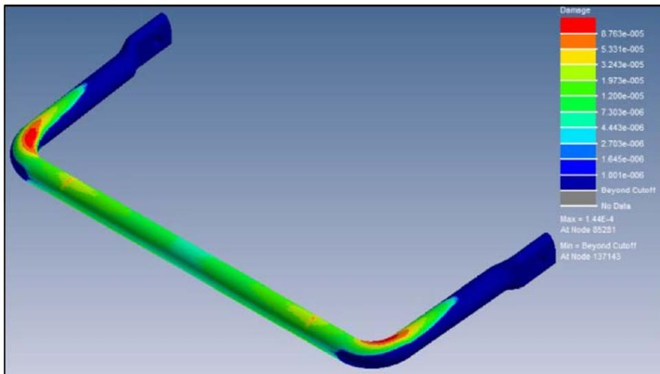
As can be noted, both bars showed a similar hotspot for damage accumulation: on their main bend. Although the different test configurations and load cases imposed different damage accumulations, the visual gradient of damage distribution has not changed on the components.
