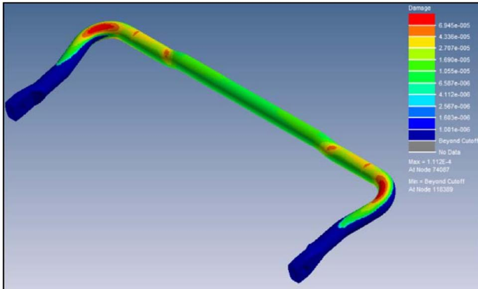
**Figure 13** SN fatigue analysis of rear anti-roll bar: soft dampers – GAWR – load case 4 (see online version for colours)
