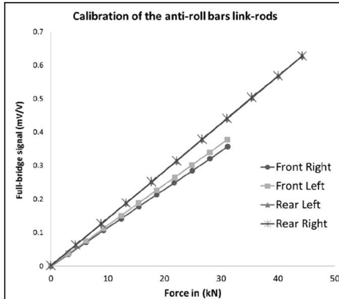
After the calibration, the link rods were assembled in the test bus and were used as dynamic load cells.
