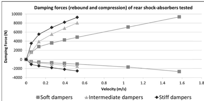
As can be noted and as discussed in Section 2.1, the shock absorbers do not present constant damping coefficients. For this reason, the term 'damping rate' is used to
