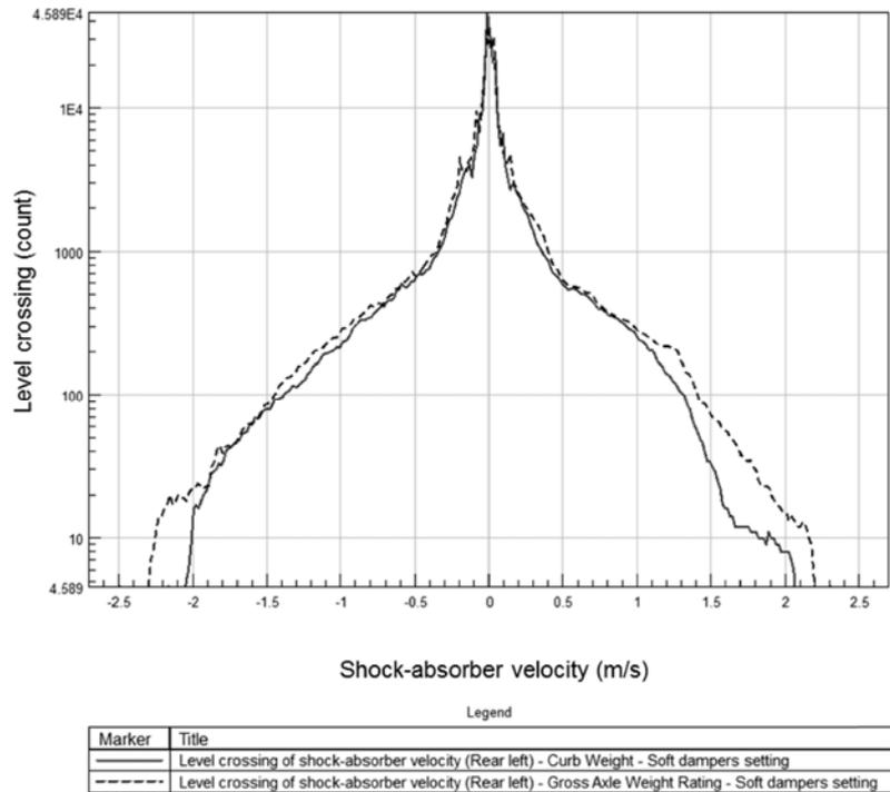
As can be noted from the histograms above, the shock absorbers reached higher peaks of velocity and presented a higher crossing count in upper speeds when tested in GAWR. At lower speeds, CW and GAWR presented very similar results. Although not presented in this work, these results could be confirmed for all shock absorbers settings (soft, intermediate and stiff) and for all positions (front left, front right, rear left and rear front).
