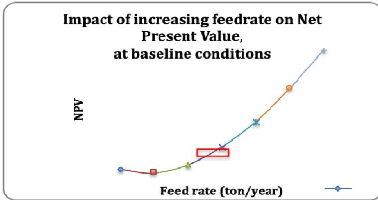
Buyback prices for electricity were incorporated into net present value calculation, at a range of \$0.07 to \$0.12 per kWh (Figure 5). At higher prices, the positive impacts can allow smaller scale designs with a feed rate of fewer than 60,000 tons per year to still be profitable.
